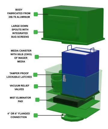
The 2050 odor control sewer valve is an elongated vertical design to accommodate a deodorizing feature that helps to suppress sewer gas odors. Perfect for residential or commercial locations where complaints regarding odor have become an issue.
