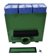
3. Unbolt water separator access plates. Inspect bolts, washers, and gasket. Remove water separator pads.
