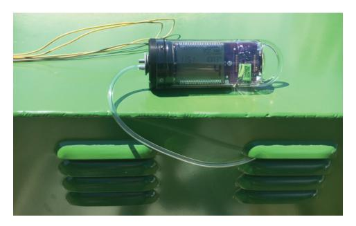
2. Place Odor Logger on top of media baskets, or place tube through the vent louvers.
