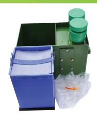
2. Ensure all of the original plastic wrap is removed from canister before reinstalling. Media is in pellet form and should move freely to allow air to vent through. To check the media, pull up on the blue tab on the media canister lid. Check that the media pellets are dry.
