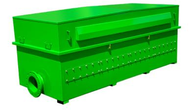
The 2050-1350 includes sixteen (16) vacuum relief valves, each capable of 300 cfm of airflow. These VRV's assure that over-pressurizing will not occur during pumping sequences on vacuum sewer systems that require additional airflow to operate. Airflow will still pass through the media bed. These vacuum relief valves simply provide additional air, but do not bypass the media bed.
