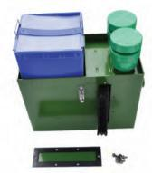
1. Unbolt water separator access plate. Inspect bolts, washers, and gasket. Remove water separator pad.
