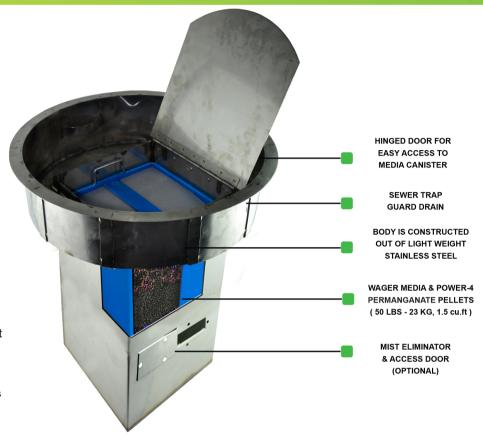
Inside the housing is one odor control canister, containing 50 lbs (23kg). of Wager media. Easy access into the Manhole Scrubber allows for quick and easy canister replacement.
