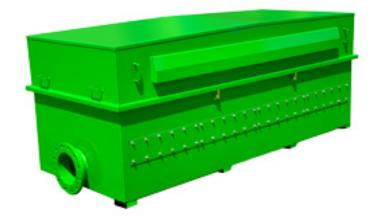
The 2050-1600 Odor Control Valve is designed to allow for ventilation and odor control at lift stations, wet wells,vaults containing ARV's and forced mains flowing into gravity fed lines. The valve is constructed from aluminum, and is epoxy coated for protection from the harsh outside environment.
