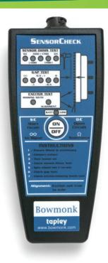
Designed with ease of use in mind, the SensorCheck takes minutes to set-up and, once connected, undertakes a complete test cycle of the six most common causes of EBS / ABS faults, at the touch of a button, in just 15 seconds - a fraction of the time it would take to perform the same tests manually - and all without having to remove the road wheel. Tests start with the continuity of the sensor and sensor lead, the status of the air gap and the condition of the exciter ring.
