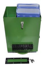
1. Unbolt water separator access plate. Inspect bolts, washers, and gasket. Remove water separator pad.
