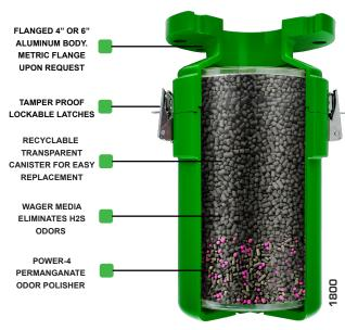
The 1800 Odor Control Vent Valve connects to a candy cane style pipe, and is designed to allow for ventilation in the open position. The valve body may be easily disassembled with two quick release lockable metal latches.
