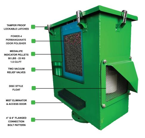
The 2050-50-IP is a combined odor control vent valve. with the additional feature of Wager's highly effective vertical vent check valve. This system is designed specifically in areas where lift stations or gravity lines are subject to flooding.
