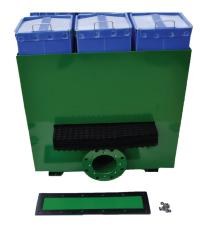
3. Unbolt water separator access plates. Inspect bolts, washers, and gasket. Remove water separator pads.
