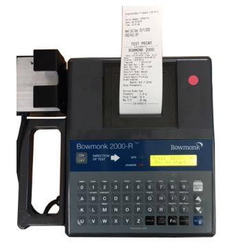
For brake testing applications, the unit will also calculate from the deceleration, time and slope, the vehicle speed at braking and distance travelled. For heavy vehicle brake testing in mines and quarries, the unit measures brake effort, which takes into account the vehicle speed and ground slope.
